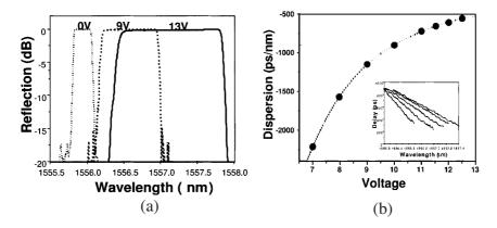
**Figure 7.17**: (a) Reflection spectrum and (b) total GVD as a function of voltage for a fiber grating with temperature gradient. Inset shows  $\tau_g(\lambda)$  at several voltages. (After Ref. [164]; ©2000 IEEE; reprinted with permission.)
