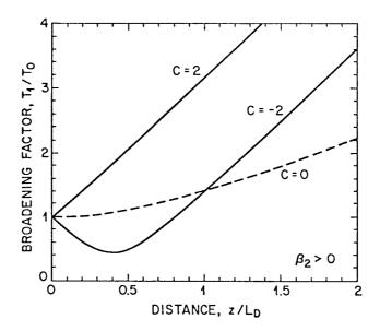
**Figure 2.12**: Variation of broadening factor with propagated distance for a chirped Gaussian input pulse. Dashed curve corresponds to the case of an unchirped Gaussian pulse. For  $\beta_2 < 0$  the same curves are obtained if the sign of the chirp parameter C is reversed.
