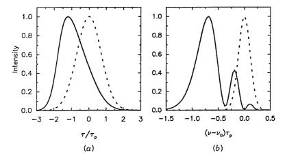
**Figure 6.9**: (a) Shape and (b) spectrum at the output of a semiconductor optical amplifier with  $G_0 = 30$  dB and  $\beta_c = 5$  for a Gaussian input pulse of energy  $E_{\rm in}/E_{\rm sat} = 0.1$ . The dashed curves show for comparison the shape and spectrum of the input pulse.
