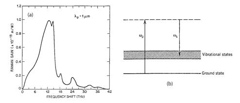
**Figure 2.18**: (a) Raman gain spectrum of fused silica at  $\lambda_p = 1 \,\mu$ m and (b) energy levels participating in the SRS process. (After Ref. [75]; © 1972 AIP; reprinted with permission.)
