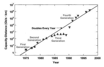
**Figure 1.4**: Increase in the BL product over the period 1975 to 1980 through several generations of lightwave systems. Different symbols are used for successive generations. (After Ref. [12]; ©2000 IEEE; reprinted with permission.)
