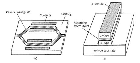
**Figure 3.27**: Two kinds of external modulators: (a) LiNbO<sub>3</sub> modulator in the Mach–Zehnder configuration; (b) semiconductor modulator based on electroabsorption.
