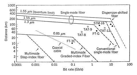
**Figure 5.4**: Loss (solid lines) and dispersion (dashed lines) limits on transmission distance L as a function of bit rate B for the three wavelength windows. The dotted line corresponds to coaxial cables. Circles denote commercial lightwave systems; triangles show laboratory experiments. (After Ref. [1]; © 1988 Academic Press; reprinted with permission.)
