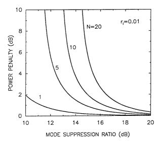
**Figure 5.14**: Feedback-induced power penalty as a function of MSR for several values of N and  $r_I = 0.01$ . Reflection feedback into the laser is assumed to generate N side modes of the same amplitude.
