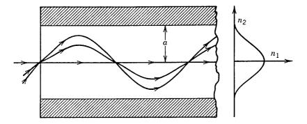
Figure 2.3: Ray trajectories in a graded-index fiber.
