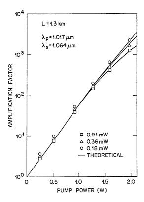
**Figure 6.12**: Variation of amplifier gain  $G_0$  with pump power  $P_0$  in a 1.3-km-long Raman amplifier for three values of the input power. Solid lines show the theoretical prediction. (After Ref. [31]; ©1981 Elsevier; reprinted with permission.)
