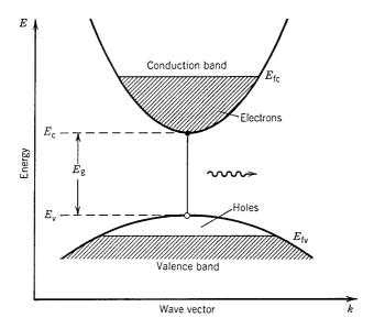
**Figure 3.2**: Conduction and valence bands of a semiconductor. Electrons in the conduction band and holes in the valence band can recombine and emit a photon through spontaneous emission as well as through stimulated emission.
