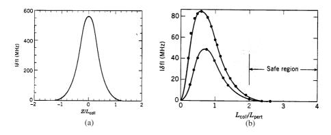
**Figure 9.26**: (a) Frequency shift during collision of two 50-ps solitons with 75-GHz channel spacing. (b) Residual frequency shift after a collision because of lumped amplifiers ( $L_A = 20$  and 40 km for lower and upper curves, respectively). Numerical results are shown by solid dots. (After Ref. [206]; ©1991 IEEE; reprinted with permission.)
