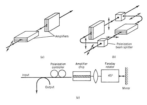
**Figure 6.6**: Three configurations used to reduce the polarization sensitivity of semiconductor optical amplifiers: (a) twin amplifiers in series; (b) twin amplifiers in parallel; and (c) double pass through a single amplifier.
