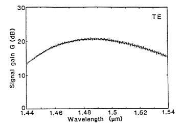
**Figure 6.5**: Amplifier gain versus signal wavelength for a semiconductor optical amplifier whose facets are coated to reduce reflectivity to about 0.04%. (After Ref. [3]; © 1987 IEEE; reprinted with permission.)
