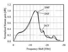
**Figure 6.11**: Raman-gain spectra (ratio  $g_R/a_p$ ) for standard (SMF), dispersion-shifted (DSF) and dispersion-compensating (DCF) fibers. Normalized gain profiles are also shown. (After Ref. [30]; ©2001 IEEE; reprinted with permission.)
