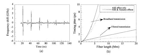
**Figure 9.24**: (a) Temporal changes in the XPM-induced frequency shift produced by acoustic waves in a 30-km-long fiber; (b) Increase in timing jitter produced by acoustic waves. (After Ref. [191]; ©2001 Academic; reprinted with permission.)
