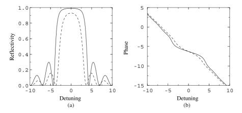
**Figure 7.8**: (a) Magnitude and (b) phase of the reflectivity plotted as a function of detuning  $\delta L_g$  for a uniform fiber grating with  $\kappa L_g = 2$  (dashed curve) or  $\kappa L_g = 3$  (solid curve).
