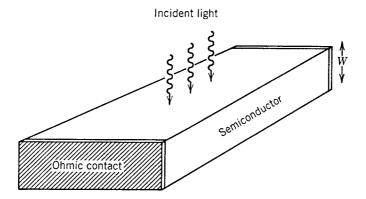
Figure 4.1: A semiconductor slab used as a photodetector.
