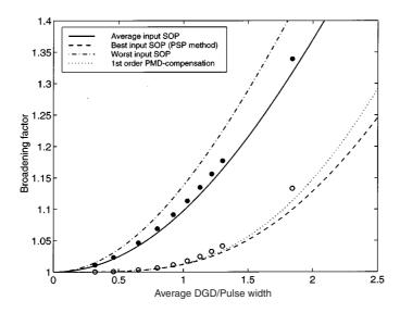
**Figure 7.22:** Pulse broadening factor as a function of average DGD in four cases. The dotted curve shows the improvement realized using a first-order PMD compensator. Filled and empty circles show the results of numerical simulations (After Ref. [206]; ©2000 IEEE; reprinted with permission.)
