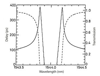
**Figure 7.10**: Transmittivity (dashed curve) and time delay (solid curve) as a function of wavelength for a uniform-pitch grating for which  $\kappa(z)$  varies linearly from 0 to 6 cm<sup>-1</sup> over the 11-cm length. (After Ref. [61]; ©1996 IEE; reprinted with permission.)
