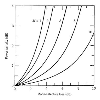
**Figure 5.6**: Modal-noise power penalty versus mode-selective loss. The parameter *M* is defined as the total number of longitudinal modes whose power exceeds 10% of the peak power. (After Ref. [61]; ©1986 IEEE; reprinted with permission.)
