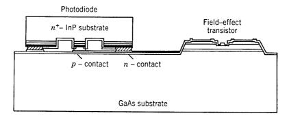
**Figure 4.14**: Flip-chip OEIC technology for integrated receivers. The InGaAs photodiode is fabricated on an InP substrate and then bonded to the GaAs chip through common electrical contacts. (After Ref. [57]; ©1988 IEE; reprinted with permission.)
