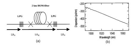
**Figure 7.5**: (a) Schematic of a DCF made using a higher-order mode (HOM) fiber and two long-period gratings (LPGs). (b) Dispersion spectrum of the DCF. (After Ref. [47]; ©2001 IEEE; reprinted with permission.)
