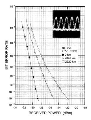
**Figure 4.24:** BER curves measured for three fiber-link lengths in a 1.55- $\mu$ m transmission experiment at 10 Gb/s. Inset shows an example of the eye diagram at the receiver. (After Ref. [110]; © 2000 IEEE; reprinted with permission.)
