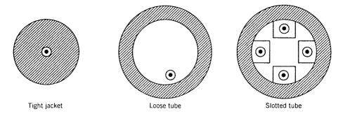
Figure 2.23: Typical designs for light-duty fiber cables.
