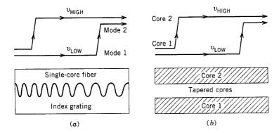
**Figure 7.13**: Schematic illustration of dispersion compensation by two fiber-based transmission filters: (a) chirped dual-mode coupler; (b) tapered dual-core fiber. (After Ref. [77]; ©1994 IEEE; reprinted with permission.)
