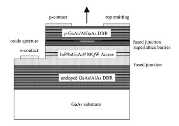
**Figure 3.19**: Schematic of a 1.55- $\mu$ m VCSEL made by using the wafer-bonding technique. (After Ref. [58]; ©2000 IEEE; reprinted with permission.)
