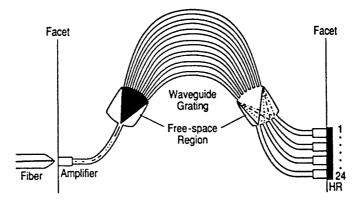
**Figure 8.21**: Schematic of a WDM laser made by integrating an AWG inside the laser cavity. (After Ref. [137]; ©1996 IEEE; reprinted with permission.)
