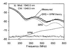
**Figure 8.31**: Predicted and measured crosstalk acquired over 25 km of fiber at 11-mW average power. The CW laser acts as a probe and its wavelength is (a) lower or (b) higher by 8.5 nm than the signal wavelength. (After Ref. [245]; ©1999 IEEE; reprinted with permission.)
