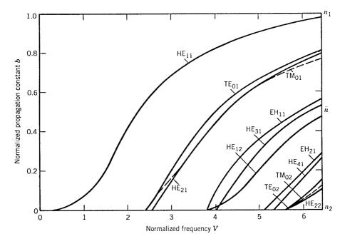
Figure 2.5: Normalized propagation constant b as a function of normalized frequency V for a few low-order fiber modes. The right scale shows the mode index  $\bar{n}$ . (After Ref. [34]; ©1981 Academic Press; reprinted with permission.)
