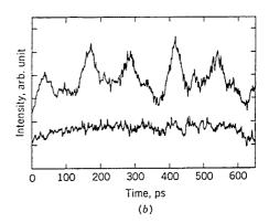
**Figure 7.3**: Streak-camera traces of the 16-Gb/s signal transmitted over 70 km of standard fiber (a) with and (b) without SOA-induced chirp. Bottom trace shows the background level in each case. (After Ref. [26]; ©1989 IEE; reprinted with permission.)
