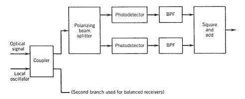
Figure 10.12: Schematic of a polarization-diversity coherent receiver.
