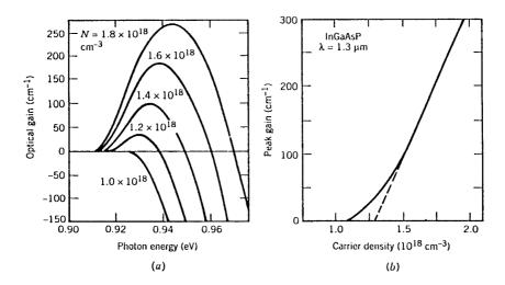
**Figure 3.9**: (a) Gain spectrum of a 1.3- $\mu$ m InGaAsP laser at several carrier densities N. (b) Variation of peak gain  $g_p$  with N. The dashed line shows the quality of a linear fit in the highgain region. (After Ref. [2]; ©1993 Van Nostrand Reinhold; reprinted with permission.)
