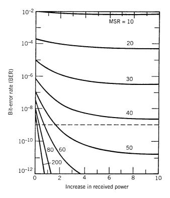
**Figure 5.9**: Effect of MPN on bit-error rate of DFB lasers for several values of MSR. Intersection of the dashed line with the solid curves provides MPN-induced power penalty. (After Ref. [85]; ©1985 IEEE; reprinted with permission.)
