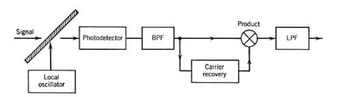
Figure 10.4: Block diagram of a synchronous heterodyne receiver.
