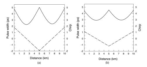
**Figure 9.16**: (a) Variations of pulse width and chirp over one map period for DM solitons with the input energy (a)  $E_0 \gg E_c = 0.1$  pJ and (b)  $E_0$  close to  $E_c$ .
