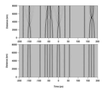
**Figure 9.20**: Propagation of a 32-bit soliton stream over 8000 km when the input pulse parameters correspond to those used in Fig. 9.16. Pulse energy equals 0.1 pJ in the top panel but has its optimum for the bottom panel.
