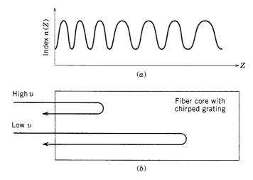
**Figure 7.11**: Dispersion compensation by a linearly chirped fiber grating: (a) index profile n(z) along the grating length; (b) reflection of low and high frequencies at different locations within the grating because of variations in the Bragg wavelength.
