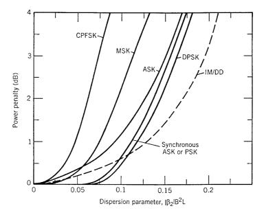
Figure 10.14: Dispersion-induced power penalty as a function of the dimensionless parameter  $|\beta_2|B^2L$  for several modulation formats. The dashed line shows power penalty for a direct-detection system. (After Ref. [95]; © 1988 IEEE; reprinted with permission.)
