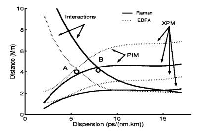
**Figure 9.29**: Maximum transmission distance as a function of local dispersion for a WDM soliton system with 40-Gb/s channels spaced apart by 100 GHz. The curves with labels "Interactions" and "XPM" show limitations due to intrachannel and interchannel pulse interactions, respectively. The PIM curves correspond to the case of polarization multiplexing. (After Ref. [248]); ©2001 OSA; reprinted with permission.)
