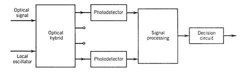
**Figure 10.9**: Schematic of a multiport phase-diversity receiver.
