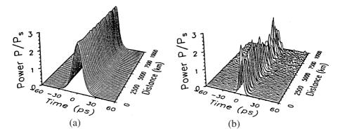
**Figure 9.11:** Evolution of loss-managed solitons over 10,000 km for (a)  $L_D = 200$  km and (b) 25 km with  $L_A = 50$  km,  $\alpha = 0.22$  dB/km, and  $\beta_2 = -0.5$  ps<sup>2</sup>/km.
