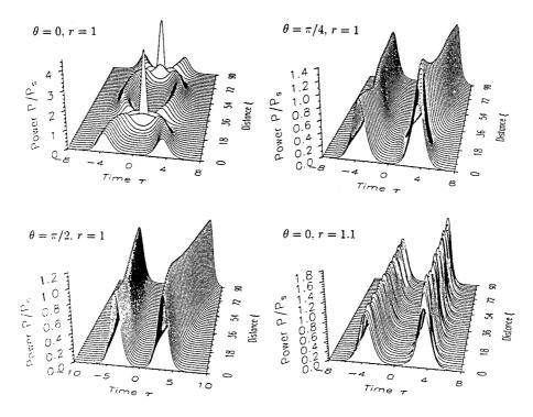
**Figure 9.6**: Evolution of a soliton pair over 90 dispersion lengths showing the effects of soliton interaction for four different choices of amplitude ratio r and relative phase  $\theta$ . Initial spacing  $q_0 = 3.5$  in all four cases.
