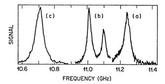
**Figure 2.17**: Brillouin-gain spectra measured using a 1.525- $\mu$ m pump for three fibers with different germania doping: (a) silica-core fiber; (b) depressed-cladding fiber; (c) dispersion-shifted fiber. Vertical scale is arbitrary. (After Ref. [78]; © 1986 IEE; reprinted with permission.)
