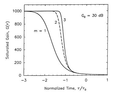
**Figure 6.7**: Time-dependent amplification factor for super-Gaussian input pulses of input energy such that  $E_{\rm in}/E_{\rm sat}=0.1$ . The unsaturated value  $G_0$  is 30 dB in all cases. The input pulse is Gaussian for m=1 but becomes nearly rectangular as m increases.
