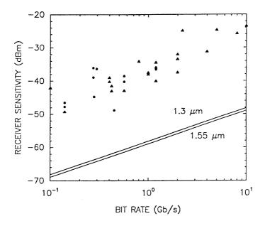
**Figure 4.23**: Measured receiver sensitivities versus the bit rate for p–i–n (circles) and APD (triangles) receivers in transmission experiments near 1.3- and 1.55- $\mu$ m wavelengths. The quantum limit of receiver sensitivity is also shown for comparison (solid lines).
