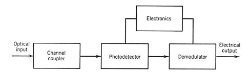
Figure 1.12: Components of an optical receiver.
