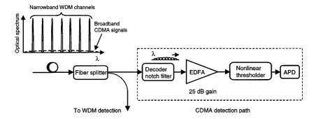
**Figure 8.34**: Receiver for a hybrid WDM–CDMA system sharing the same spectral bandwidth. A notch filter is used within the decoder to remove the WDM signal. (After Ref. [267]; ©2001 IEEE; reprinted with permission.)
