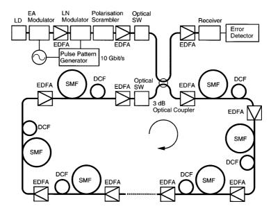
**Figure 7.15**: Recirculating fiber loop used to demonstrate transmission of a 10-Gb/s signal over 10,000 km of standard fiber using a DCF periodically. Components used include laser diode (LD), electroabsorption (EA) modulator, optical switch (SW), fiber amplifier (EDFA), single-mode fiber (SMF), and DCF. (After Ref. [135]; ©2000 IEEE; reprinted with permission.)
