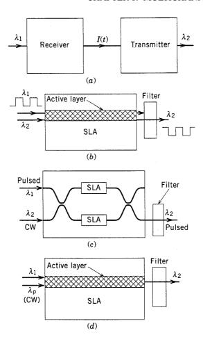
**Figure 8.20**: Four schemes for wavelength conversion: (a) optoelectronic regenerator; (b) gain saturation in a semiconductor laser amplifier (SLA); (c) phase modulation in a SLA placed in one arm of a Mach-Zehnder interferometer; (d) four-wave mixing inside a SLA.
