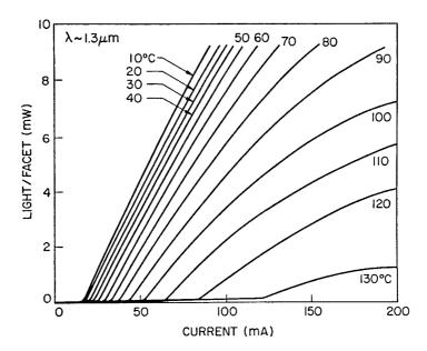
**Figure 3.20**: P-I curves at several temperatures for a 1.3- $\mu$ m buried heterostructure laser. (After Ref. [2]; ©1993 Van Nostrand Reinhold; reprinted with permission.)
