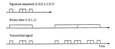
**Figure 8.32**: Coding of binary data in CDM systems using a signature sequence in the form of a 7-chip code.
