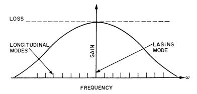
**Figure 3.11**: Gain and loss profiles in semiconductor lasers. Vertical bars show the location of longitudinal modes. The laser threshold is reached when the gain of the longitudinal mode closest to the gain peak equals loss.
