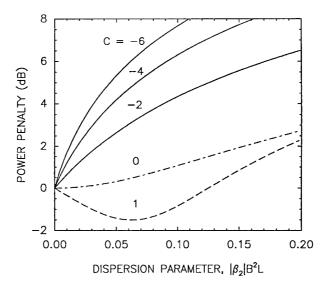
**Figure 5.11:** Chirp-induced power penalty as a function of  $|\beta_2|B^2L$  for several values of the chirp parameter C. The Gaussian optical pulse is assumed to be linearly chirped over its entire width.
