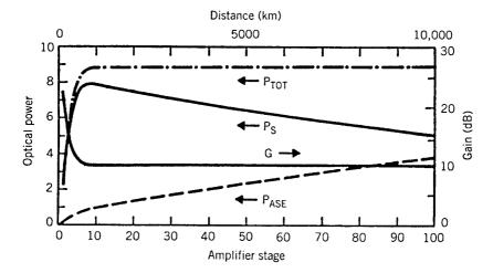
**Figure 6.21**: Variation of the signal power  $P_s$  and the ASE power  $P_{ASE}$  along a cascaded chain of optical amplifiers. The total power  $P_{TOT}$  becomes nearly constant after a few amplifiers. (After Ref. [119]; ©1991 IEEE; reprinted with permission.)
