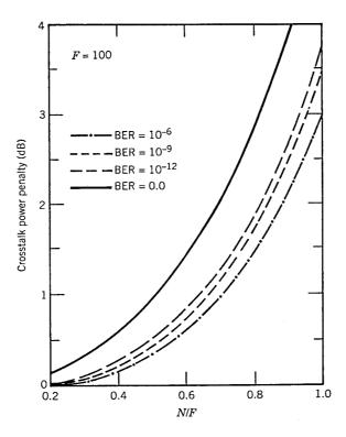
Figure 8.22: Crosstalk power penalty at four different values of the BER for a FP filter of finesse F = 100. (After Ref. [149]; ©1990 IEEE; reprinted with permission.)
