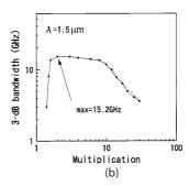
**Figure 4.10**: (a) Device structure and (b) measured 3-dB bandwidth as a function of M for a superlattice APD. (After Ref. [38]; ©2000 IEEE; reprinted with permission.)
