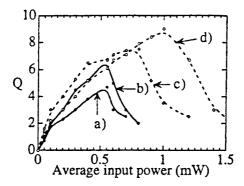
**Figure 6.24**: *Q* factor as a function of the average input power for a 9000-km fiber link: (a) 5-Gb/s system; (b) improvement realized with 150-GHz optical filters; (c) 6-Gb/s operation near the zero-dispersion wavelength; (d) 10-Gb/s system with dispersion management. (After Ref. [134]; ©1996 IEEE; reprinted with permission.)
