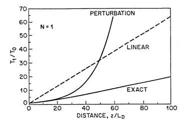
**Figure 9.9**: Broadening of fundamental solitons in lossy fibers ( $\Gamma = 0.07$ ). The curve marked "exact" shows numerical results. Dashed curve shows the behavior expected in the absence of nonlinear effects. (After Ref. [55]; ©1985 Elsevier; reprinted with permission.)
