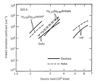
**Figure 4.7**: Impact-ionization coefficients of several semiconductors as a function of the electric field for electrons (solid line) and holes (dashed line). (After Ref. [24]; ©1977 Elsevier; reprinted with permission.)
