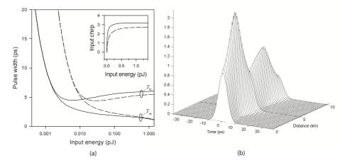
**Figure 9.15**: (a) Changes in  $T_0$  (upper curve) and  $T_m$  (lower curve) with input pulse energy  $E_0$  for  $\alpha = 0$  (solid lines) and 0.25 dB/km (dashed lines). The inset shows the input chirp  $C_0$  in the two cases. (b) Evolution of the DM soliton over one map period for  $E_0 = 0.1$  pJ and  $L_A = 80$  km.
