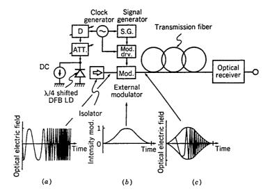
**Figure 7.1**: Schematic of the prechirp technique used for dispersion compensation: (a) FM output of the DFB laser; (b) pulse shape produced by external modulator; and (c) prechirped pulse used for signal transmission. (After Ref. [9]; ©1994 IEEE; reprinted with permission.)
