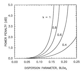
**Figure 5.8**: MPN-induced Power penalty versus  $BLD\sigma_{\lambda}$  for a multimode semiconductor laser of RMS spectral width  $\sigma_{\lambda}$ . Different curves correspond to different values of the mode-partition coefficient k.
