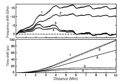
**Figure 9.28**: Collision-induced frequency and temporal shifts for a soliton surrounded by four channels on each side (75 GHz spacing). Curves 1 and 2 represent the case copolarized and orthogonally polarized solitons in neighboring channels, respectively. Curves 3 and 4 show the improvement realized with sliding-frequency filters. The dotted line shows the prediction of an analytical model. (After Ref. [238]); ©1999 OSA; reprinted with permission.)
