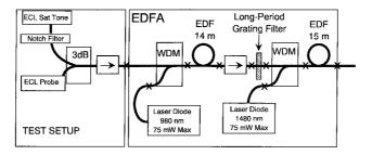
**Figure 6.18**: Schematic of an EDFA designed to provide uniform gain over the 1530–1570-nm bandwidth using an optical filter containing several long-period fiber gratings. The two-stage design helps to reduce the noise level. (After Ref. [85]; ©1997 IEEE; reprinted with permission.)
