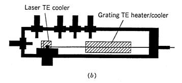
**Figure 9.8**: Schematic of (a) the device and (b) the package for a hybrid soliton pulse source. (After Ref. [41]; ©1995 IEEE; reprinted with permission.)
