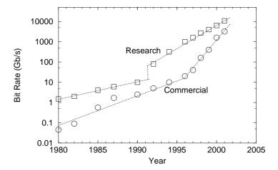
**Figure 1.3**: Increase in the capacity of lightwave systems realized after 1980. Commercial systems (circles) follow research demonstrations (squares) with a few-year lag. The change in the slope after 1992 is due to the advent of WDM technology.
