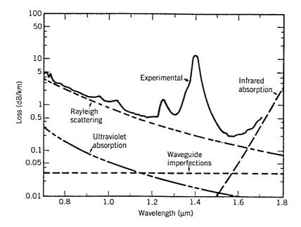
**Figure 2.15**: Loss spectrum of a single-mode fiber produced in 1979. Wavelength dependence of several fundamental loss mechanisms is also shown. (After Ref. [11]; ©1979 IEE; reprinted with permission.)
