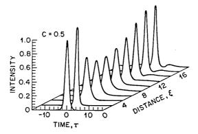
Figure 9.7: Evolution of a chirped optical pulse for the case N = 1 and C = 0.5. For C = 0 the pulse shape does not change, since the pulse propagates as a fundamental soliton.
