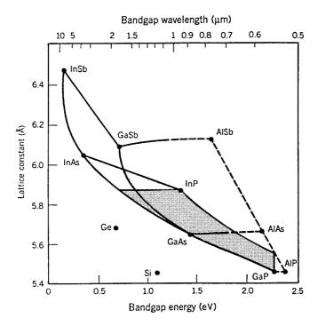
**Figure 3.5**: Lattice constants and bandgap energies of ternary and quaternary compounds formed by using nine group III–V semiconductors. Shaded area corresponds to possible InGaAsP and AlGaAs structures. Horizontal lines passing through InP and GaAs show the lattice-matched designs. (After Ref. [18]; ©1991 Wiley; reprinted with permission.)
