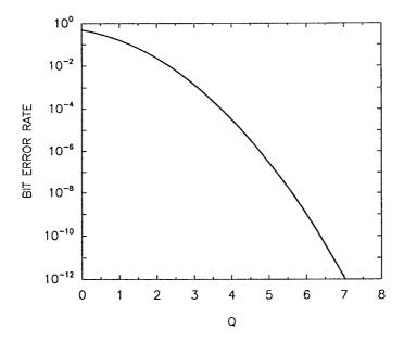
**Figure 4.19**: Bit-error rate versus the *Q* parameter.
