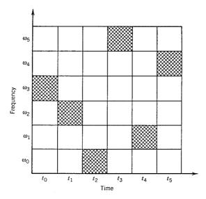
**Figure 8.33**: Frequency hopping in CDM lightwave systems. Filled square show frequencies for different time slots. A specific frequency-hop sequence (3, 2, 0, 5, 1, 4) is shown.
