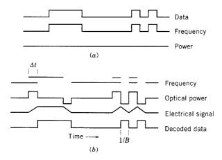
**Figure 7.2**: Dispersion compensation using FSK coding: (a) Optical frequency and power of the transmitted signal; (b) frequency and power of the received signal and the electrically decoded data. (After Ref. [13]; ©1994 IEEE; reprinted with permission.)
