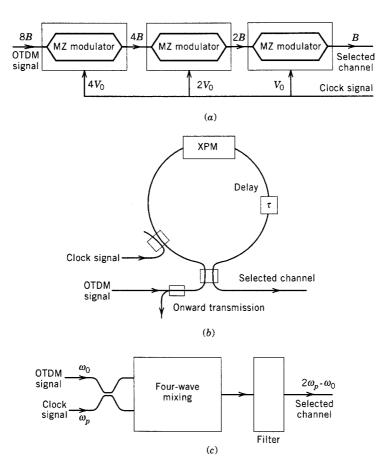
**Figure 8.27**: Demultiplexing schemes for OTDM signals based on (a) cascaded LiNbO<sub>3</sub> modulators, (b) XPM in a nonlinear optical-loop mirror, and (c) FWM in a nonlinear medium.
