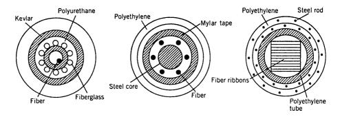
**Figure 2.24**: Typical designs for heavy-duty fiber cables.
