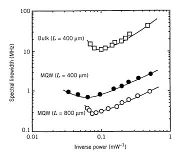
**Figure 3.24**: Measured linewidth as a function of emitted power for several 1.55- $\mu$ m DFB lasers. Active layer is 100 nm thick for the bulk laser and 10 nm thick for MQW lasers. (After Ref. [86]; ©1991 IEEE; reprinted with permission.)
