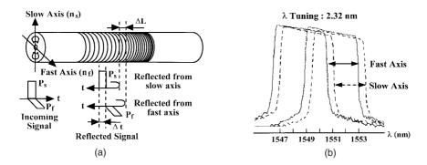
**Figure 7.21**: Tunable PMD compensation provided by a birefringent chirped fiber grating. (a) The origin of differential group delay; (b) stop-band shift induced by stretching the grating. (After Ref. [160]; ©1999 IEEE; reprinted with permission.)
