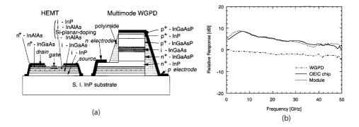
**Figure 4.15**: (a) Epitaxial-layer structure and (b) frequency response of an OEIC receiver module made using a waveguide photodetector (WGPD). (After Ref. [73]; ©2000 IEEE; reprinted with permission.)
