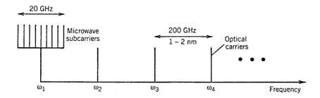
**Figure 8.30**: Frequency allocation in a multiwavelength SCM network.
