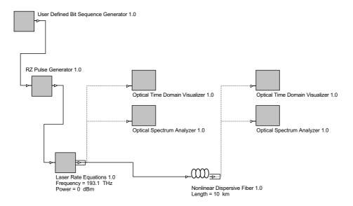
**Figure E.1:** An example of the layout for studying the propagation of optical pulses inside optical fibers. All the components are available in the standard component library supplied with the OptiSystem Lite software.
