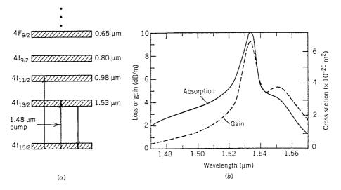
**Figure 6.15**: (a) Energy-level diagram of erbium ions in silica fibers; (b) absorption and gain spectra of an EDFA whose core was codoped with germania. (After Ref. [64]; ©1991 IEEE; reprinted with permission.)
