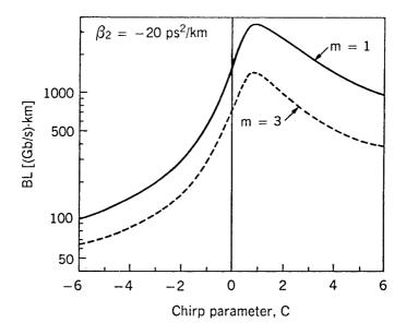
**Figure 2.14**: Dispersion-limited *BL* product as a function of the chirp parameter for Gaussian (solid curve) and super-Gaussian (dashed curve) input pulses. (After Ref. [58]; ©1986 OSA; reprinted with permission.)
