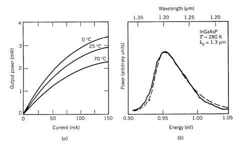
**Figure 3.7**: (a) Power–current curves at several temperatures; (b) spectrum of the emitted light for a typical 1.3- $\mu$ m LED. The dashed curve shows the theoretically calculated spectrum. (After Ref. [21]; ©1983 AT&T; reprinted with permission.)
