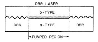
**Figure 3.16**: DFB and DBR laser structures. The shaded area shows the active region and the wavy line indicates the presence of a Bragg gratin.
