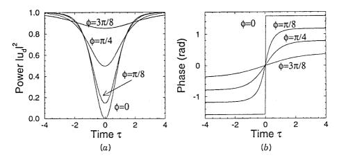
**Figure 9.4**: (a) Intensity and (b) phase profiles of dark solitons for several values of the internal phase  $\phi$ . The intensity drops to zero at the center for black solitons.
