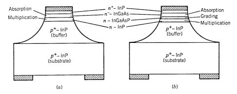
Figure 4.9: Design of (a) SAM and (b) SAGM APDs containing separate absorption, multiplication, and grading regions.
