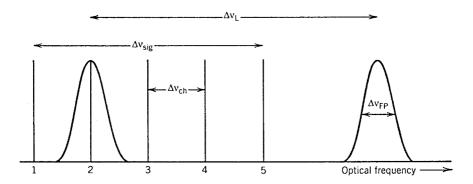
Figure 8.7: Channel selection through a tunable optical filter.
