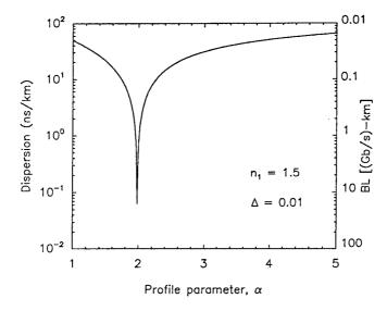
**Figure 2.4**: Variation of intermodal dispersion  $\Delta T/L$  with the profile parameter  $\alpha$  for a graded-index fiber. The scale on the right shows the corresponding bit rate–distance product.
