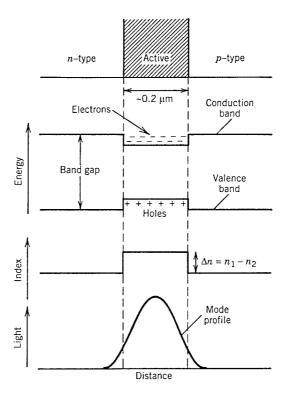
**Figure 3.4:** Simultaneous confinement of charge carriers and optical field in a double-heterostructure design. The active layer has a lower bandgap and a higher refractive index than those of *p*-type and *n*-type cladding layers.
