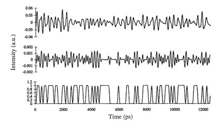
**Figure 8.25**: XPM-induced power fluctuations on a CW probe for a 130-km link (middle) and a 320-km link (top) with dispersion management. An NRZ bit stream in the pump channel is shown at the bottom. (After Ref. [191], ©1999 IEEE; reprinted with permission.)
