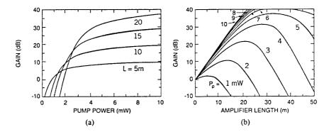
**Figure 6.16**: Small-signal gain as a function of (a) pump power and (b) amplifier length for an EDFA assumed to be pumped at 1.48  $\mu$ m. (After Ref. [64]; ©1991 IEEE; reprinted with permission.)
