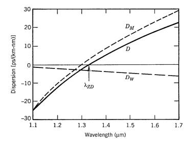
**Figure 2.10**: Total dispersion D and relative contributions of material dispersion  $D_M$  and waveguide dispersion  $D_W$  for a conventional single-mode fiber. The zero-dispersion wavelength shifts to a higher value because of the waveguide contribution.
