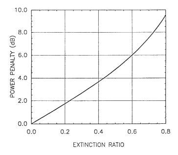
**Figure 4.20**: Power penalty versus the extinction ratio  $r_{\rm ex}$ .
