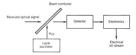
Figure 10.1: Schematic illustration of a coherent detection scheme.
