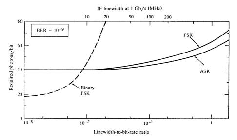
**Figure 10.8**: Receiver sensitivity  $\bar{N}_p$  versus  $\Delta v/B$  for asynchronous ASK and FSK heterodyne receivers. The dashed line shows the sensitivity degradation for a synchronous PSK heterodyne receiver. (After Ref. [49]; ©1988 IEEE; reprinted with permission.)
