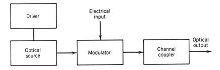
Figure 1.11: Components of an optical transmitter.
