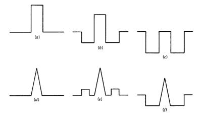
**Figure 2.20**: Several index profiles used in the design of single-mode fibers. Upper and lower rows correspond to standard and dispersion-shifted fibers, respectively.
