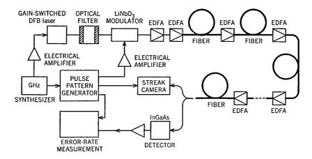
**Figure 9.13**: Setup used for soliton transmission in a 1990 experiment. Two EDFAs after the LiNbO<sub>3</sub> modulator boost pulse peak power to the level of fundamental solitons. (After Ref. [70]; © 1990 IEEE; reprinted with permission.)
