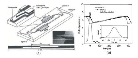
**Figure 8.28**: (a) Mach–Zehnder TOAD demultiplexer with two SOAs placed asymmetrically. Insets show the device structure. (b) Gain variations inside two SOAs and the resulting switching window. (After Ref. [225]; ©2001 IEEE; reprinted with permission.)
