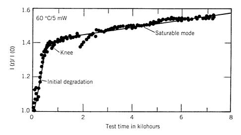
**Figure 3.28**: Change in current as a function of time for a 1.3- $\mu$ m InGaAsP laser aged at 60°C with 5 mW of output power. (After Ref. [148]; ©1985 AT&T; reprinted with permission.)
