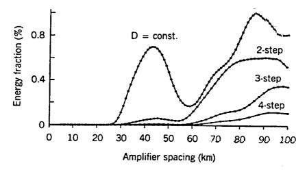
**Figure 9.27**: Fraction of soliton energy in an FWM sideband during a single collision when the exponential GVD profile is approximated by a staircase with two, three, and four steps. The case of constant-dispersion fibers is shown for comparison. (After Ref. [222]); ©1996 OSA; reprinted with permission.)
