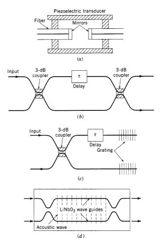
**Figure 8.8**: Four kinds of filters based on various interferometric and diffractive devices: (a) Fabry–Perot filter; (b) Mach–Zehnder filter; (c) grating-based Michelson filter; (d) acousto-optic filter. The shaded area represents a surface acoustic wave.
