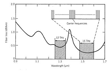
**Figure 8.1:** Low-loss transmission windows of silica fibers in the wavelength regions near 1.3 and 1.55  $\mu$ m. The inset shows the WDM technique schematically.
