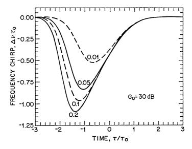
**Figure 6.8**: Frequency chirp imposed across the amplified pulse for several values of  $E_{\rm in}/E_{\rm sat}$ . A Gaussian input pulse is assumed together with  $G_0 = 30$  dB and  $\beta_c = 5$ . (After Ref. [19]; ©1989 IEEE; reprinted with permission.)
