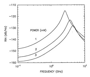
**Figure 3.23**: RIN spectra at several power levels for a typical  $1.55-\mu m$  semiconductor laser.
