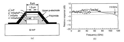
**Figure 4.6**: (a) Schematic cross section of a mushroom-mesa waveguide photodiode and (b) its measured frequency response. (After Ref. [17]; © 1994 IEEE; reprinted with permission.)
