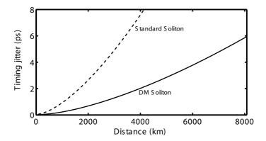
**Figure 9.17**: (a) ASE-induced timing jitter as a function of length for a 40-Gb/s system designed with DM (solid curve) and standard (dashed line) solitons.
