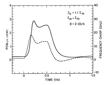
**Figure 3.22**: Simulated modulation response of a semiconductor laser to 500-ps rectangular current pulses. Solid curve shows the pulse shape and the dashed curve shows the frequency chirp imposed on the pulse ( $\beta_c = 5$ ).
