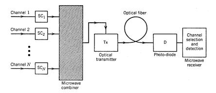
**Figure 8.29**: Schematic illustration of subcarrier multiplexing. Multiple microwave subcarriers (SC) are modulated, and the composite electrical signal is used to modulate an optical carrier at the transmitter (Tx).
