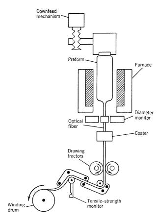
Figure 2.22: Apparatus used for fiber drawing.
