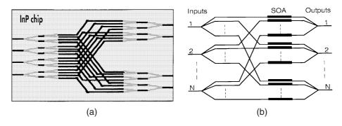
**Figure 8.19**: Examples of optical switches based on (a) Y-junction semiconductor waveguides and (b) SOAs with splitters. (After Ref. [105]; ©1996 IEEE; reprinted with permission.)
