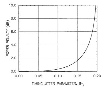
**Figure 4.22**: Power penalty versus the timing jitter parameter  $B\tau_i$ .
