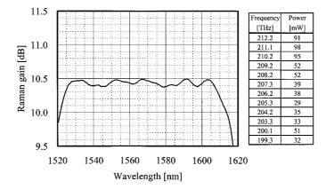
**Figure 6.14**: Measured gain profile of a Raman amplifier with nearly flat gain over an 80-nm bandwidth. Pump frequencies and powers used are shown on the right. (After Ref. [30]; ©2001 IEEE; reprinted with permission.)
