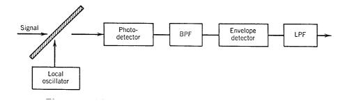
**Figure 10.5**: Block diagram of an asynchronous heterodyne receiver.
