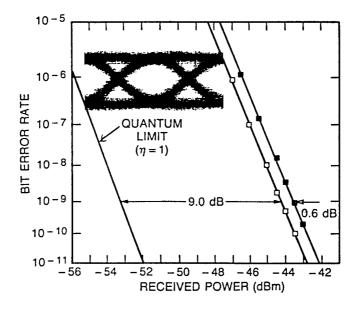
**Figure 10.15**: BER curves for a 4-Gb/s PSK homodyne transmission experiment with 5 m (empty squares) and 167 km (filled squares) of fiber. The quantum limit is shown for comparison. The inset shows the eye diagram after 167 km of fiber at −44 dBm received power. (After Ref. [145]; ©1990 IEEE; reprinted with permission.)
