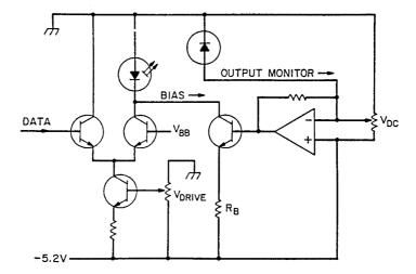
**Figure 3.26**: Driving circuit for a laser transmitter with feedback control to keep the average optical power constant. A photodiode monitors the output power and provides the control signal. (After Ref. [95]; ©1988 Academic Press; reprinted with permission.)
