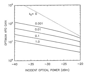
**Figure 4.17**: Optimum APD gain  $M_{\text{opt}}$  as a function of the incident optical power  $P_{\text{in}}$  for several values of  $k_A$ . Parameter values corresponding to a typical 1.55- $\mu$ m InGaAs APD receiver were used.
