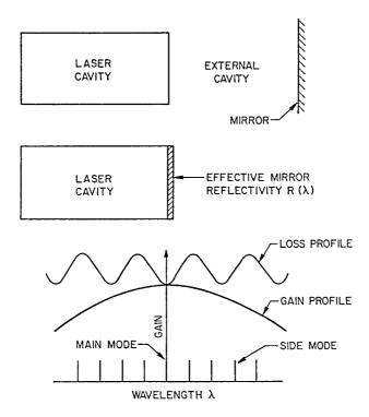
**Figure 3.17**: Longitudinal-mode selectivity in a coupled-cavity laser. Phase shift in the external cavity makes the effective mirror reflectivity wavelength dependent and results in a periodic loss profile for the laser cavity.
