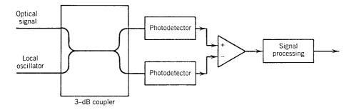
Figure 10.11: Schematic of a two-port balanced coherent receiver.
