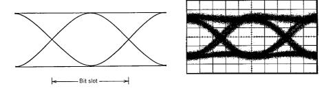
Figure 4.13: Ideal and degraded eye patterns for the NRZ format.
