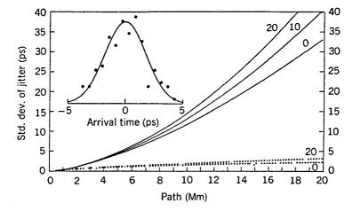
**Figure 9.18**: Timing jitter with (dotted curves) and without (solid curves) sliding-frequency filters at several bit rates as a function of distance. The inset shows a Gaussian fit to the numerically simulated jitter at 10,000 km for a 10-Gb/s system. (After Ref. [129]; ©1992 OSA; reprinted with permission.)
