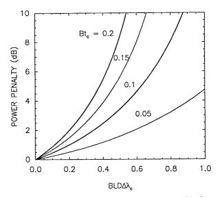
**Figure 5.10**: Chirp-induced power penalty as a function of  $BLD\Delta\lambda_c$  for several values of the parameter  $Bt_c$ , where  $\Delta\lambda_c$  is the wavelength shift occurring because of frequency chirp and  $t_c$  is the duration of such a wavelength shift.
