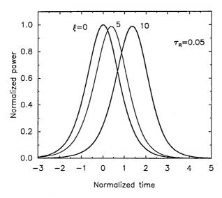
Figure 9.22: Pulse envelopes at distances  $\xi = z/L_D = 0$ , 5, and 10 showing the delay of a soliton because of the Raman-induced-frequency shift.
