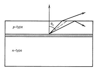
**Figure 3.6**: Total internal reflection at the output facet of an LED. Only light emitted within a cone of angle  $\theta_c$  is transmitted, where  $\theta_c$  is the critical angle for the semiconductor—air interface.
