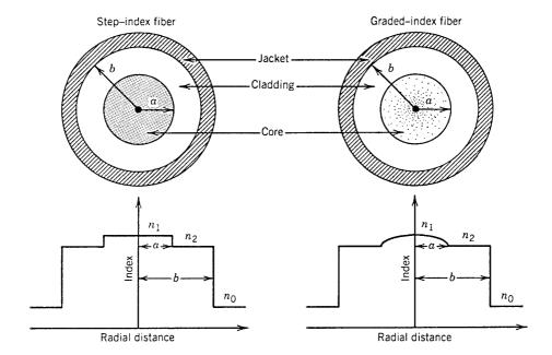
Figure 2.1: Cross section and refractive-index profile for step-index and graded-index fibers.
